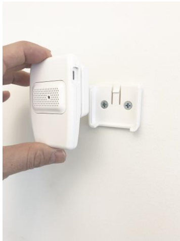
2. Slide the Sensor into the Mounting Bracket on the wall.
